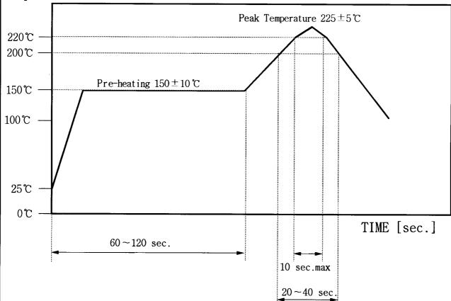
The standard condition of reflow soldering temperature and time is shown in the above. When the reflow soldering may be repeated, the maximum time must be the accumulated total time.
