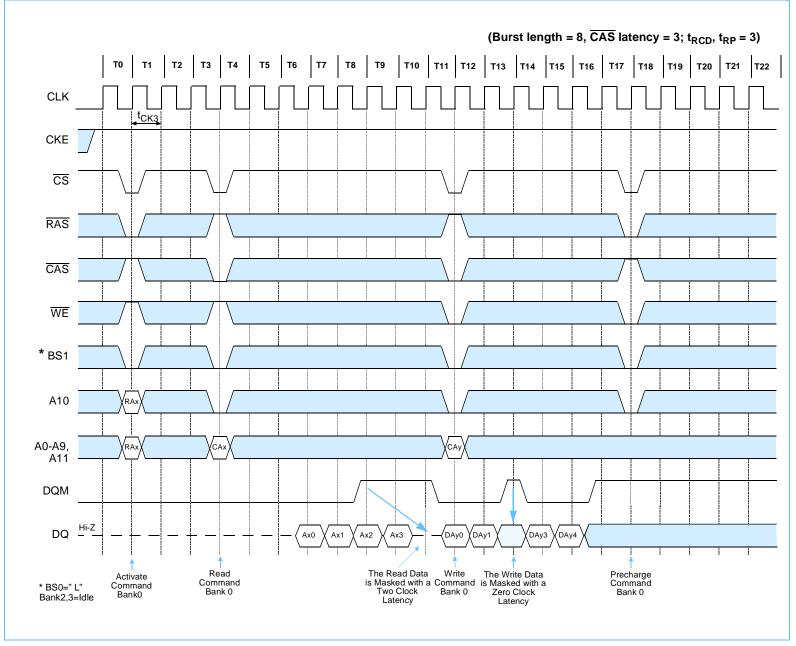
Interleaved Column Read Cycle
