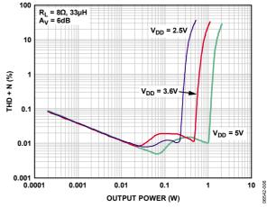
Figure 6. THD + N vs. Output Power into 8  $\Omega$ ,  $A_V = 6 dB$
