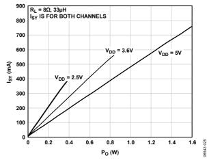
Figure 25. Supply Current vs. Output Power into 8  $\Omega$
