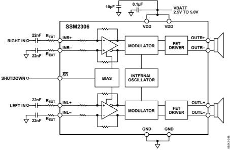
Figure 33. Stereo Single-Ended Input Configuration
