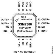
Figure 2. Pin Configuration
