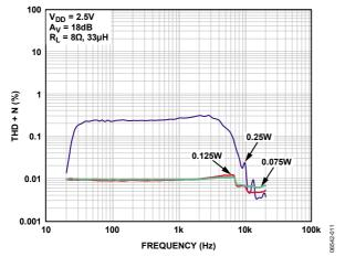
Figure 11. THD + N vs. Frequency,  $V_{DD} = 2.5 \text{ V}$ ,  $R_L = 8 \Omega$ ,  $A_V = 18 \text{ dB}$
