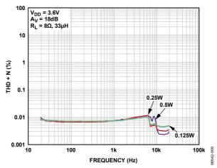
Figure 9. THD + N vs. Frequency,  $V_{DD} = 3.6 \text{ V}$ ,  $R_L = 8 \Omega$ ,  $A_V = 18 \text{ dB}$
