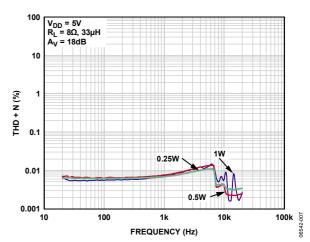
Figure 7. THD + N vs. Frequency,  $V_{DD} = 5 V$ ,  $R_L = 8 \Omega$ ,  $A_V = 18 dB$
