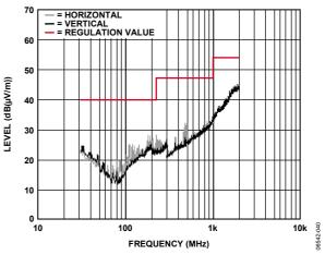
Figure 35. EMI Emissions from SSM2306
