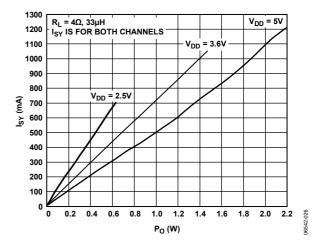
Figure 26. Supply Current vs. Output Power into 4  $\Omega$
