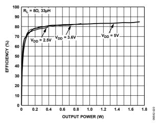
Figure 20. Efficiency vs. Output Power into 8  $\Omega$
