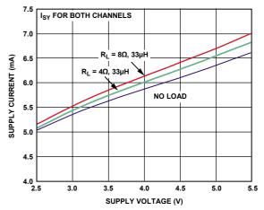
Figure 13. Supply Current vs. Supply Voltage, No Load
