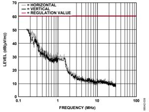
Figure 34. EMI Emissions from SSM2306
