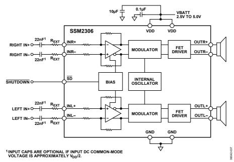
Figure 32. Stereo Differential Input Configuration
