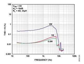
Figure 8. THD + N vs. Frequency,  $V_{DD}$  = 5 V,  $R_L$  = 4  $\Omega$ ,  $A_V$  = 18 dB
