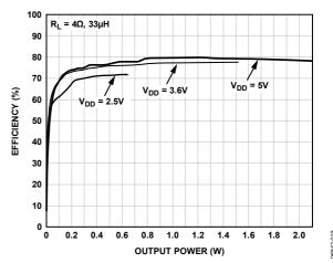
Figure 19. Efficiency vs. Output Power into 4  $\Omega$
