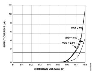
Figure 14. Supply Current vs. Shutdown Voltage
