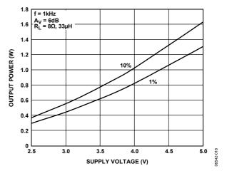
Figure 18. Maximum Output Power vs. Supply Voltage,  $R_L = 8 \Omega$ ,  $A_V = 6 dB$
