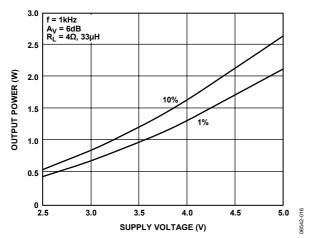
Figure 16.Maximum Output Power vs. Supply Voltage,  $R_L = 4 \Omega$ ,  $A_V = 6 dB$
