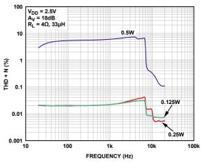
Figure 12. THD + N vs. Frequency,  $V_{DD}$  = 2.5 V,  $R_L$  = 4  $\Omega$ ,  $A_V$  = 18 dB
