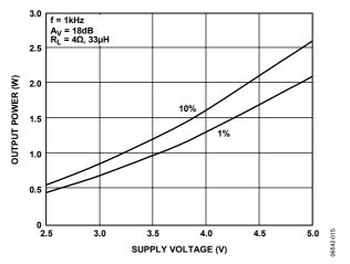
Figure 15. Maximum Output Power vs. Supply Voltage,  $R_L = 4 \Omega$ ,  $A_V = 18 dB$
