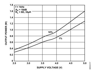
Figure 17. Maximum Output Power vs. Supply Voltage,  $R_L = 8 \Omega$ ,  $A_V = 18 dB$
