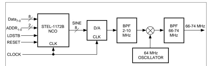
If the STEL-1172B is combined with a high-speed 8-bit video DAC, signals with spectral purity of better than -55 dBc can be generated up to 10 MHz. In this way a signal can be generated in the 66 to 74 MHz band after filtering and upconversion. Because of the phase continuous frequency switching characteristics of the STEL-1172B this architecture is suitable for Frequency Hopping Spread Spectrum applications.
