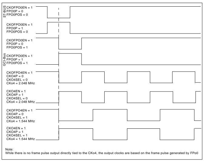
Figure 11 - Output Timing for CKo4
