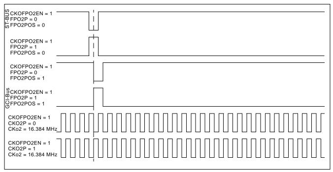
Figure 9 - Output Timing for CKo2 and FPo2
