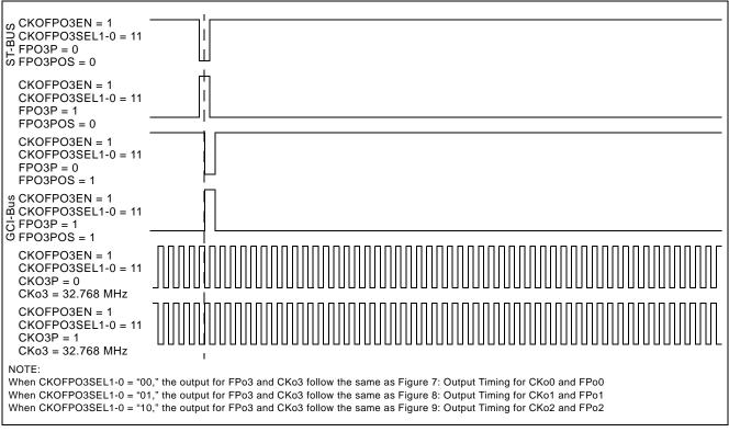
Figure 10 - Output Timing for CKo3 and FPo3 with CK0FPo3SEL1-0="11"
