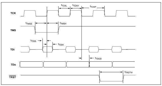
Figure 28 - JTAG Test Port Timing Diagram
