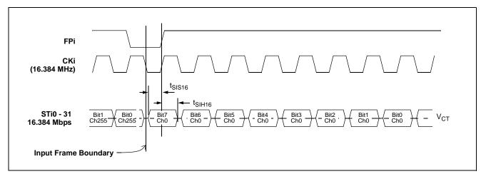
Figure 32 - ST-BUS Input Timing Diagram when Operated at 16 Mbps
