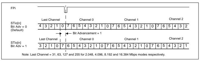
Figure 16 - Output Bit Advancement Timing Diagram (ST-BUS)
