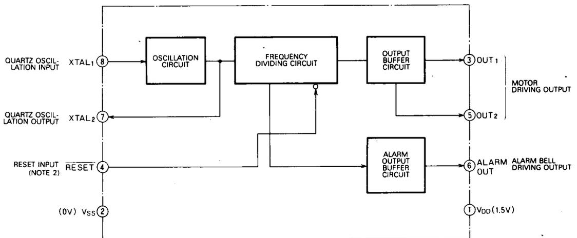
Note 2: M58434P has no reset input pin.
