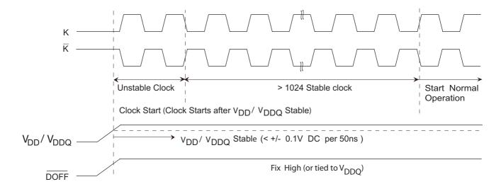
14. It is recommended that the DOFF pin be pulled HIGH via a pull up resistor of 1 Kohm.
