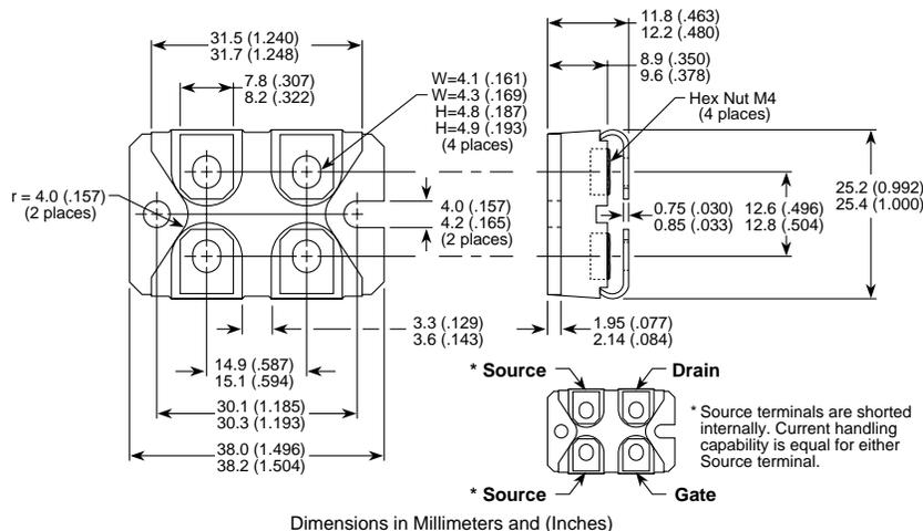
\* Source terminals are shorted internally. Current handling capability is equal for either Source terminal.
