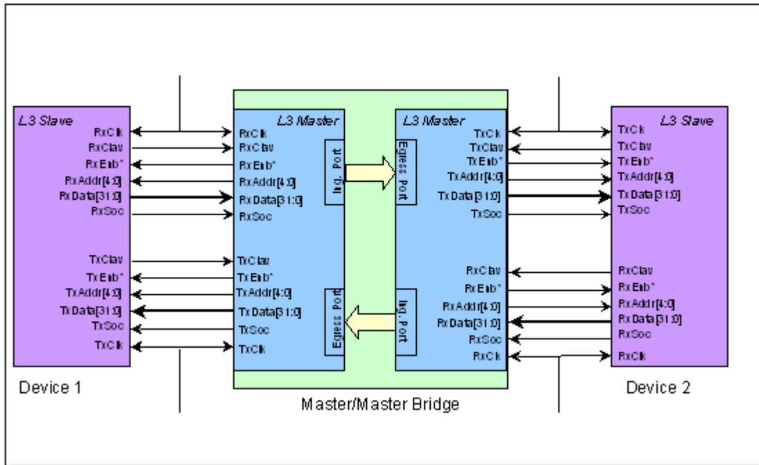
Figure 3: Master/Master Bridge connecting two Slave Devices
