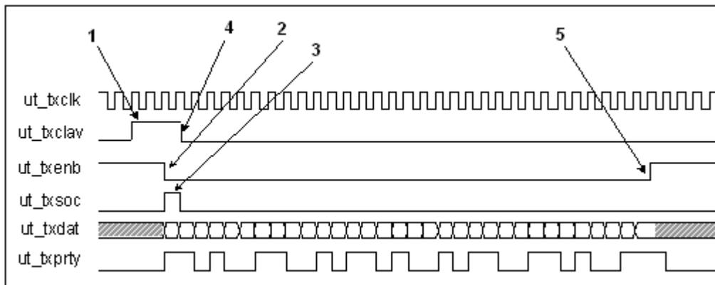
Figure 6: Single Cell Transfer - Cell Level Transfer
