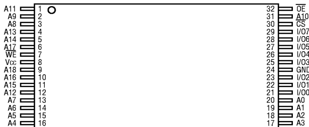
32 TSOP (REVERSE) TOP VIEW
