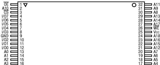
32 TSOP (REVERSE) TOP VIEW
