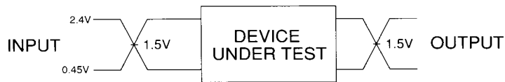
A.C. testing, inputs are driven at 2.4V for a logic "1" and .45V for a logic "0". Input and output timing measurements are made at 1.5V for both a logic "1" and "0".
