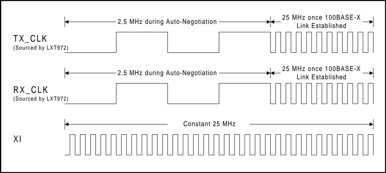
Figure 10: Link Down Clock Transition
