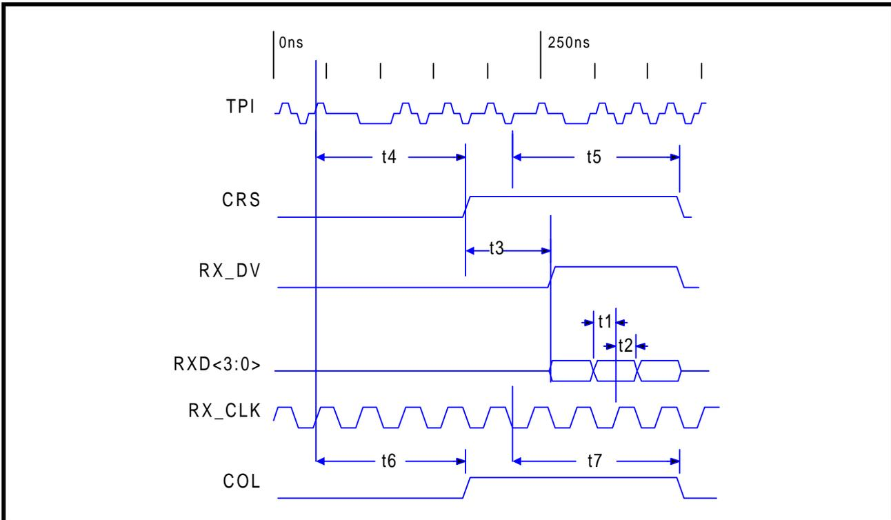
Table 25: 100BASE-TX Receive Timing Parameters - 4B Mode
