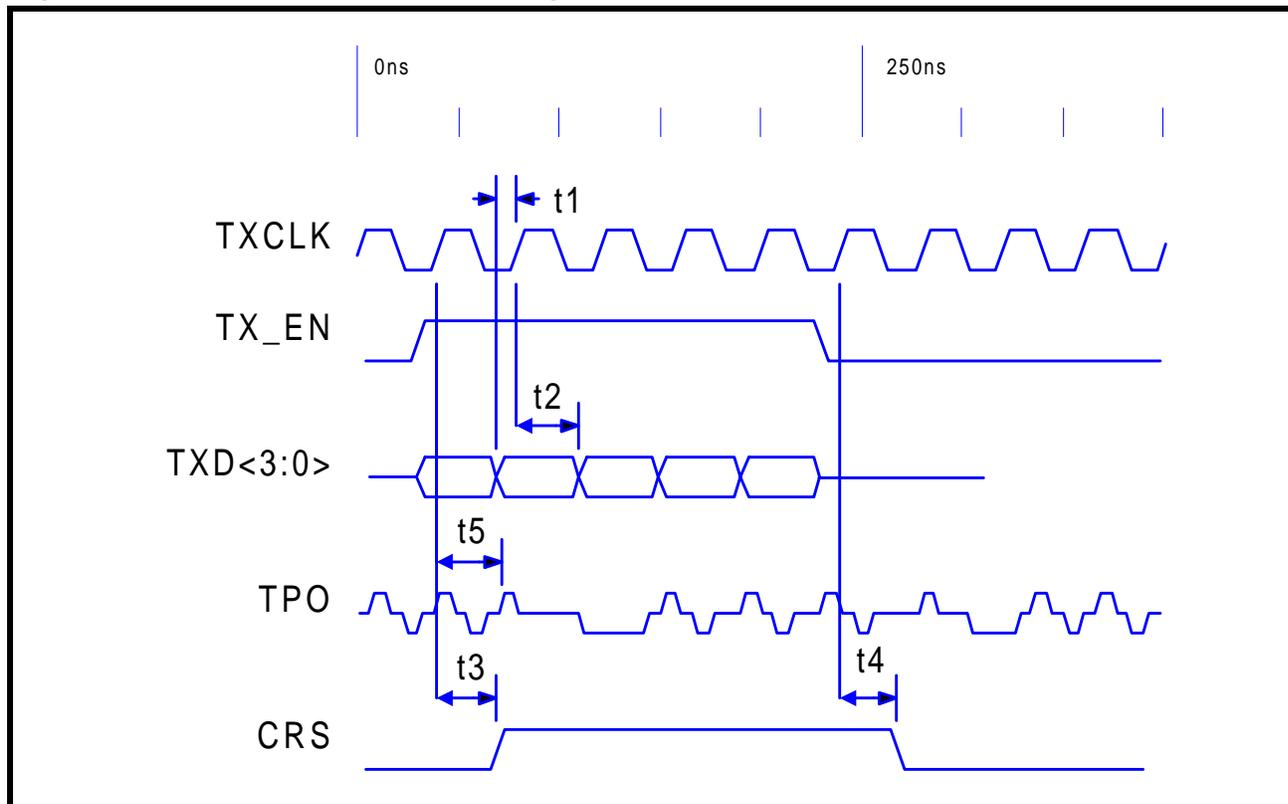
Table 26: 100BASE-TX Transmit Timing Parameters - 4B Mode
