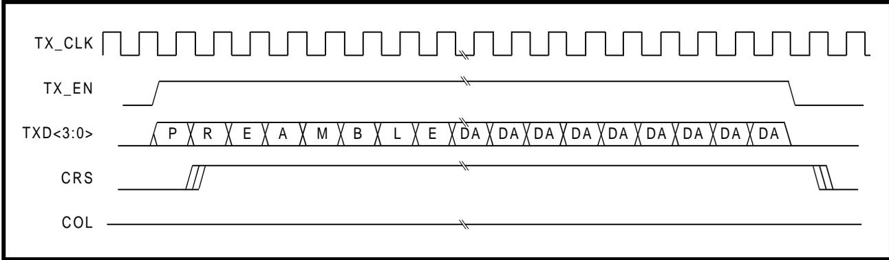
Figure 17: 100BASE-TX Transmission with Collision
