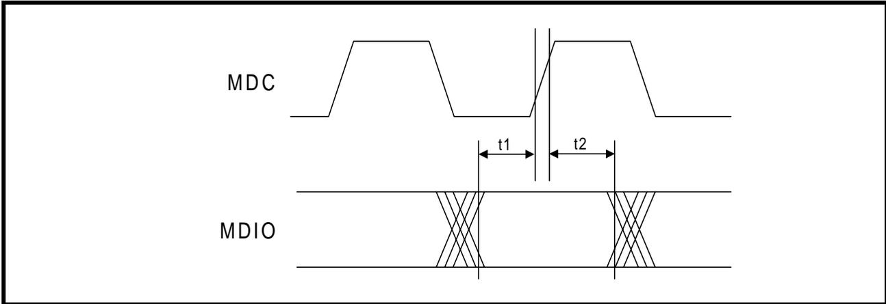
Figure 32: MDIO Output Timing
