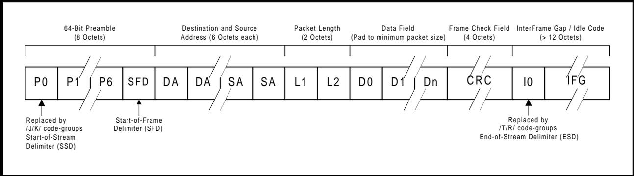
Figure 13: 100BASE-TX Data Path
