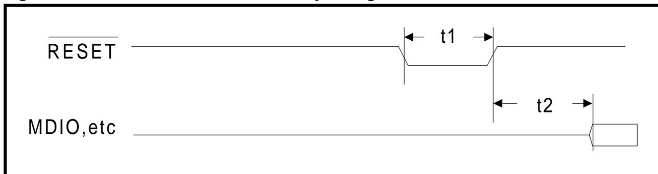
Table 34:  $\overline{\text{RESET}}$  Pulse Width and Recovery Timing Parameters
