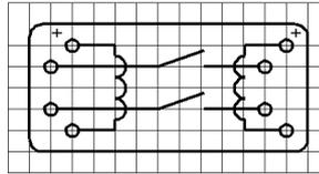
Coil polarity must be observed.
