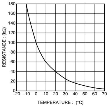
Fig.6 Thermistor curve
