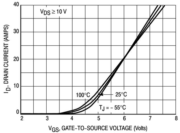
Figure 2. Transfer Characteristics
