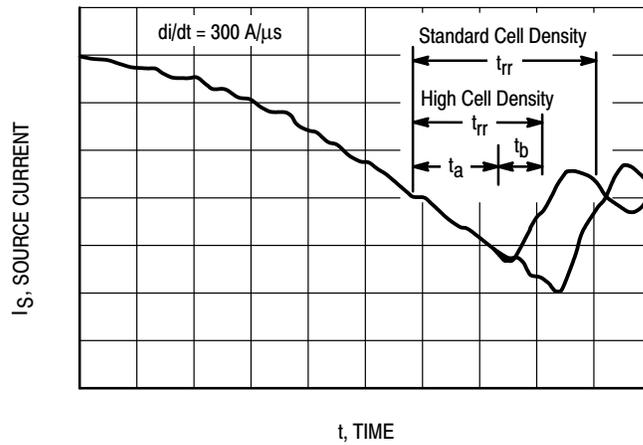
Figure 10. Reverse Recovery Time ( $t_{rr}$ )
