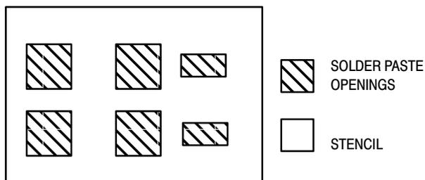
Figure 16. Typical Stencil for DPAK and D<sup>2</sup>PAK Packages
