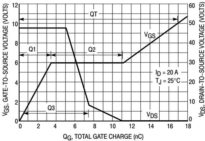
Figure 7. Gate-To-Source and Drain-To-Source Voltage versus Total Charge
