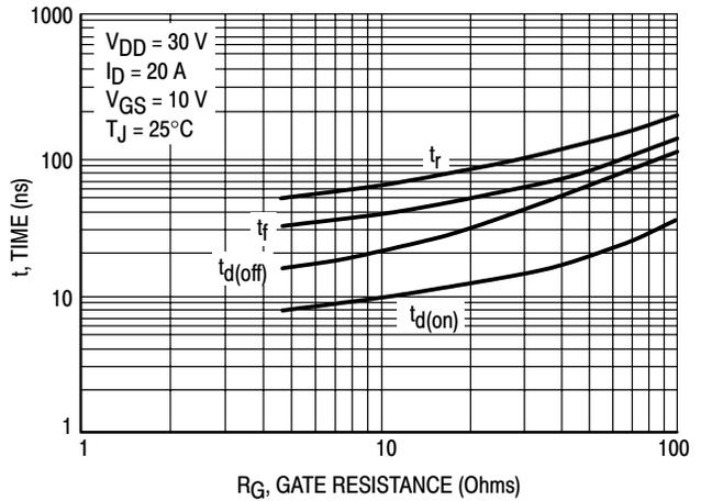
Figure 8. Resistive Switching Time Variation versus Gate Resistance
