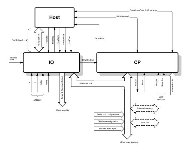
The IO chip contains the parallel host interface, the incremental encoder input along with pulse and direction motor output signals.
