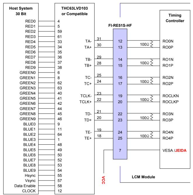
Note :1. The LCD module uses a 100  $Ohm[\Omega]$  resistor between positive and negative lines of each receiver input
