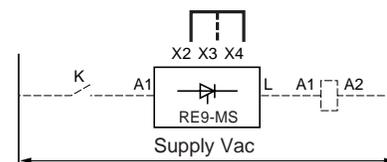
Link to be made between terminals X2 and X4.
