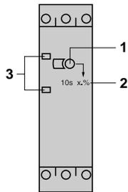
**NOTE:** For supply voltages greater than 30 V, the rated voltage of the load is equal to the supply voltage. For a supply voltage of 24 V, the voltage drop within the RE9 timer must be taken into account (about 3 V); a coil with a nominal voltage of 21 V must therefore be selected for the load.
