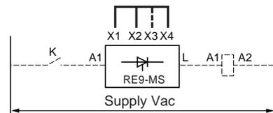
Link to be made between terminals X2 and X4 on one side and X1 and X2 on the other side.
