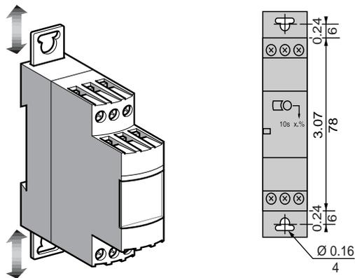
Dual Dimensions =  $\frac{\text{in}}{\text{mm}}$
