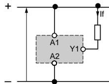
Leakage current (open state) if < 1 mA.
