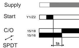
External control for partial stop of time delay (example on pulse on energization relay) RE7ML, MY
