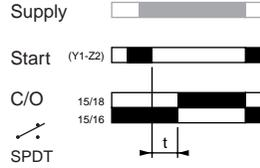
External Control for Partial Stop of Time Delay (for totalizing function) **RE7TM**
