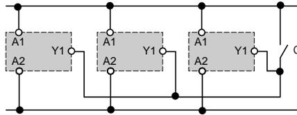
The external control contact C may be an electronic control device, for example a 2-wire sensor. In this case A1-A2 = 24 Vdc and the control device can only control up to a maximum of 4 timers.
