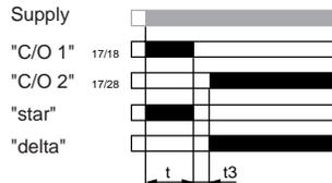
External control for start of time delay (example on On-delay function) RE7ML, MY
