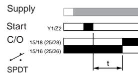
Interval Timer with Start on Opening of the External Control Contact RE7ML, MY
