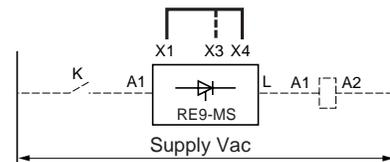
Link to be made between terminals X1 and X4.
