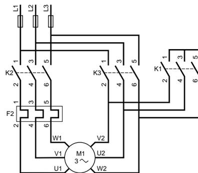
Control Wiring "Star-Delta" function with interval contact for "Star" operation
