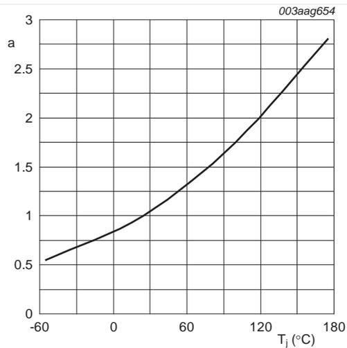
$$a = \frac{R_{DS(on)}}{R_{DS(on)(25^\circ\text{C})}}$$
