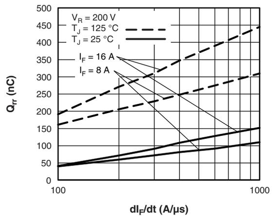
Fig. 8 - Typical Stored Charge vs.  $di_F/dt$
