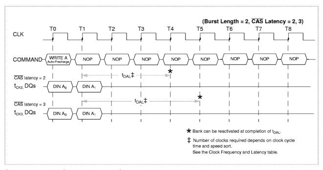
Similar to the Read Command, a Write Command with auto-precharge can not be interrupted by a command to the same bank. It can be interrupted by a Read or Write Command to a different bank, however. The precharge function will be initiated by the new command. After the Data-in to Active, delay,  $t_{DAL}$ , is satisfied the bank may be reactivated.
