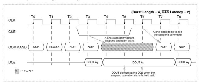
If Clock Suspend mode is initiated during a burst write operation, the input data is masked and is ignored until the Clock Suspend mode is exited.
