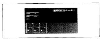
Located in the left part of the display is the indicator area, this indicates the various program steps to the user, as well as the display units in 1/min or 1/sec during operation, and the status of output signals
