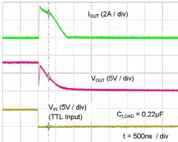
Figure 43. Quasi-Static Sink Current with  $V_{DD}=8V$ <sup>(13)</sup>
