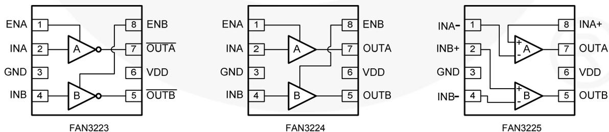
Figure 1. Pin Configurations
