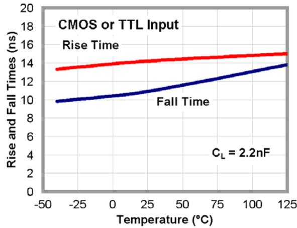
Figure 37. Rise and Fall Times vs. Temperature
