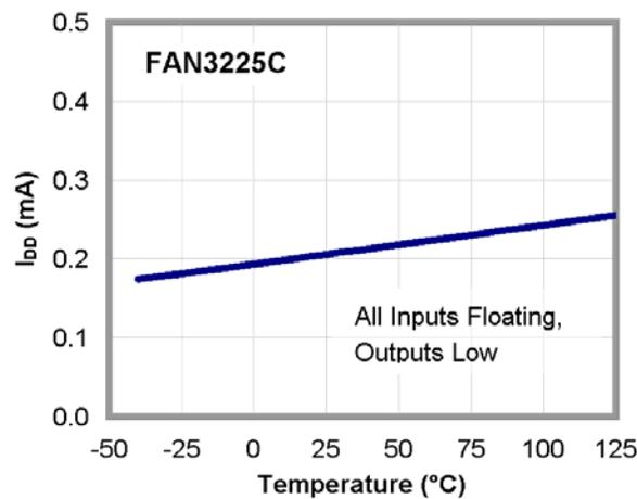
Figure 19.  $I_{DD}$  (Static) vs. Temperature<sup>(12)</sup>
