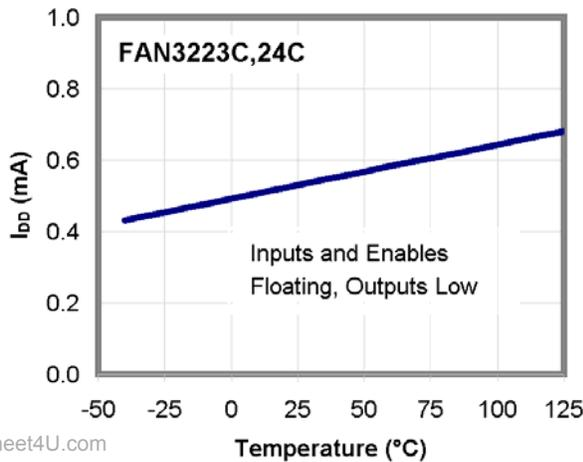
Figure 17.  $I_{DD}$  (Static) vs. Temperature<sup>(12)</sup>
