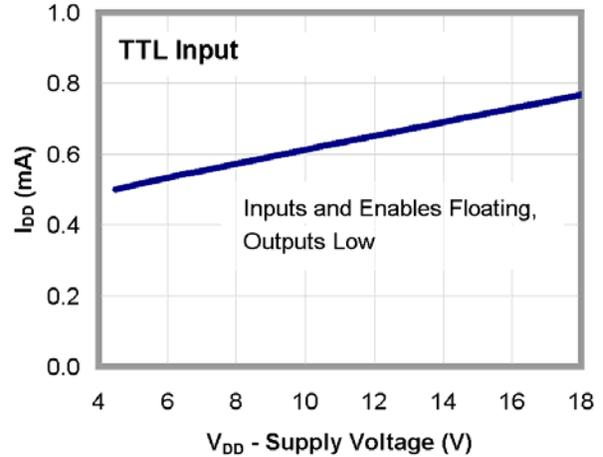
Figure 11.  $I_{DD}$  (Static) vs. Supply Voltage<sup>(12)</sup>
