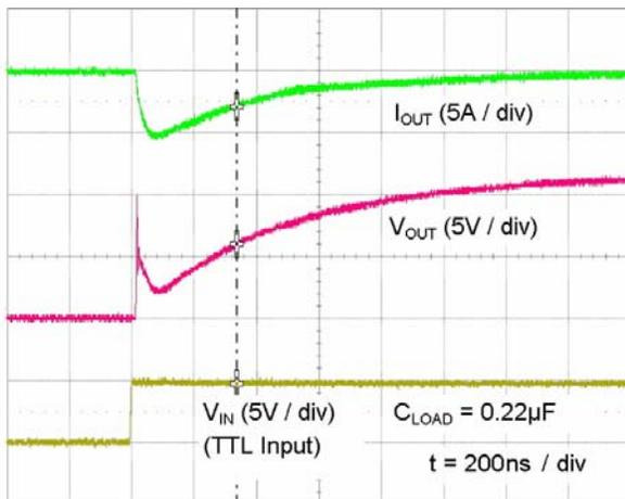
Figure 40. Quasi-Static Source Current with  $V_{DD}=12V^{(13)}$
