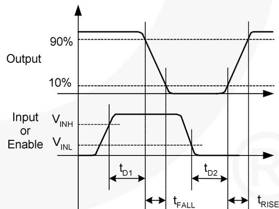
**Figure 9. Inverting**
