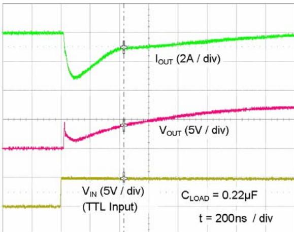
Figure 42. Quasi-Static Source Current with  $V_{DD}=8V$ <sup>(13)</sup>
