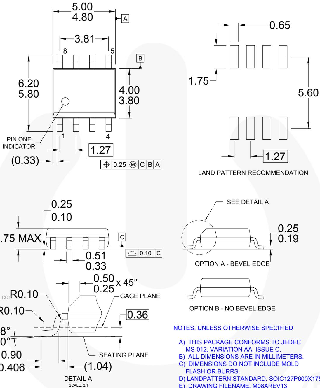
**Figure 56. 8-Lead SOIC**
