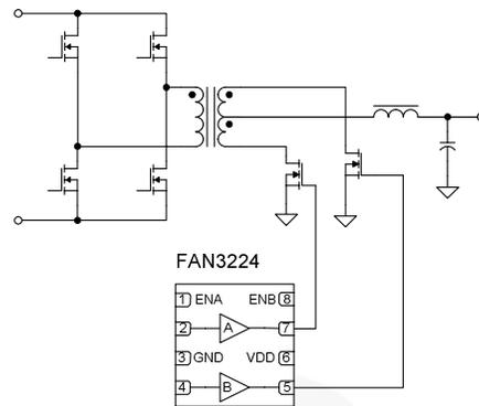
Figure 53. Center-tapped Bridge Output with Synchronous Rectifiers
