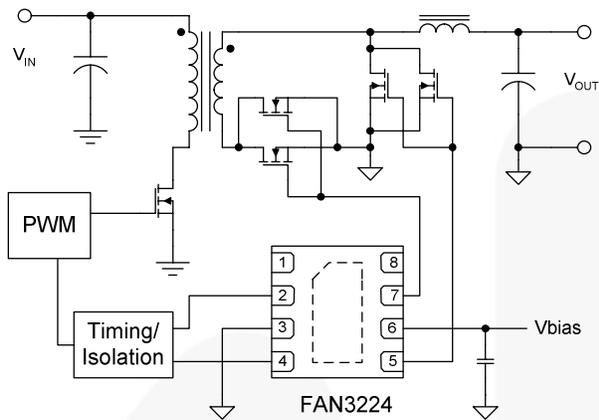
Figure 52. High Current Forward Converter with Synchronous Rectification
