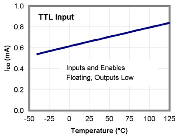
Figure 18.  $I_{DD}$  (Static) vs. Temperature<sup>(12)</sup>
