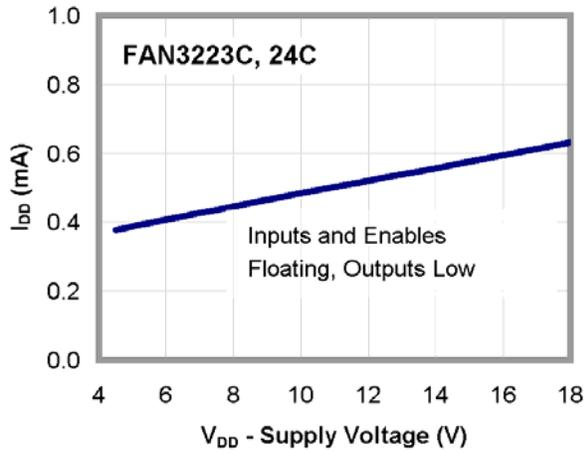
Figure 10.  $I_{DD}$  (Static) vs. Supply Voltage<sup>(12)</sup>
