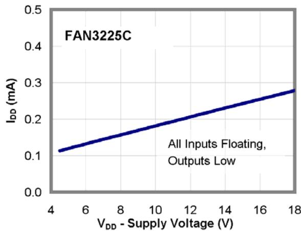
Figure 12.  $I_{DD}$  (Static) vs. Supply Voltage<sup>(12)</sup>
