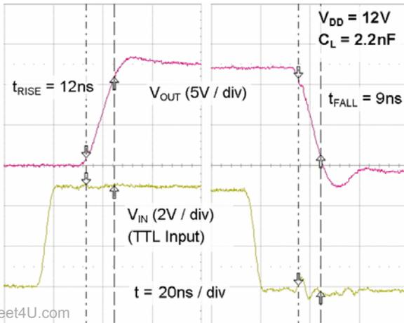
Figure 38. Rise/Fall Waveforms with 2.2nF Load
