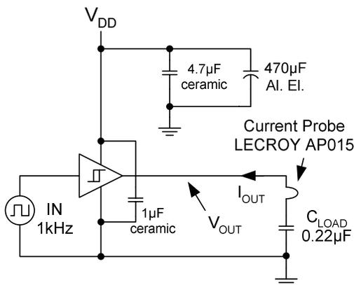
Figure 44. Quasi-Static  $I_{OUT}$  /  $V_{OUT}$  Test Circuit
