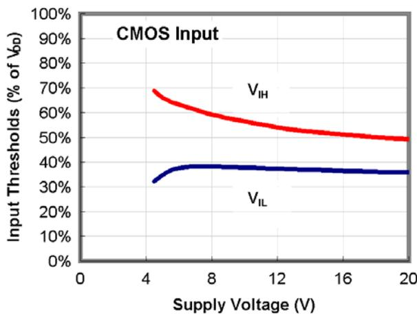
Figure 22. Input Threshold % vs. Supply Voltage
