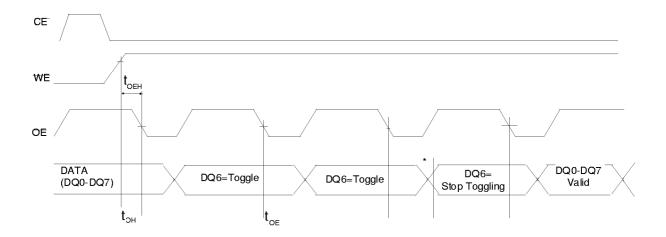
\* DQ6 stops toggling ( the device has completed the embedded operations)
