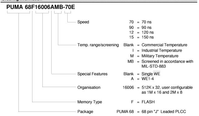
NOTE: The E variant is designated to parts with extended Erase/Write Cycle Endurance (100,000 Min.). If not specified when ordered only a Erase/Write Cycle Endurance of 10,000 Minimum can be guaranteed.
