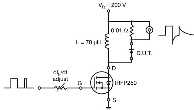
Fig. 11 - Reverse Recovery Parameter Test Circuit
