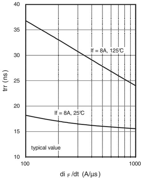
Fig. 9 - Typical Reverse Recovery vs.  $di_F/dt$
