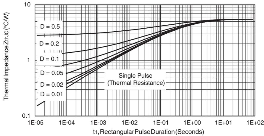
Fig. 5 - Maximum Thermal Impedance  $Z_{thJC}$  Characteristics (FULL-PAK)
