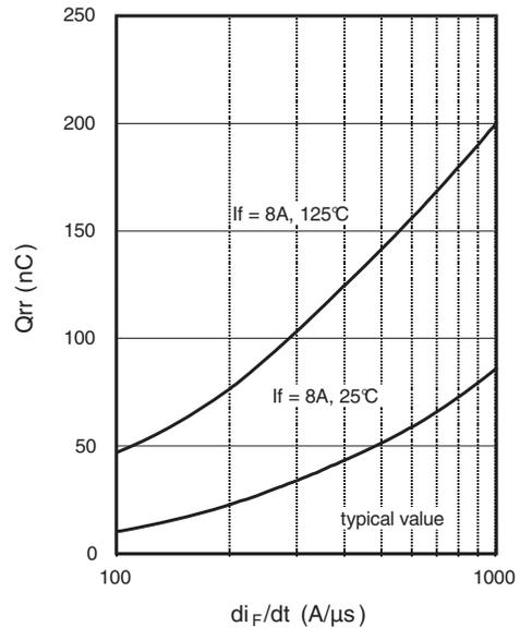
Fig. 10 - Typical Stored Charge vs.  $di_F/dt$
