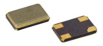
The XT35 is a miniature SMD crystal with  $5.0 \times 3.2$  (mm) ceramic package and a height of 0.8 mm. 12 MHz to 25 MHz frequncy makes it widely applied in PDA, GPS, MP3, and portable instruments.
