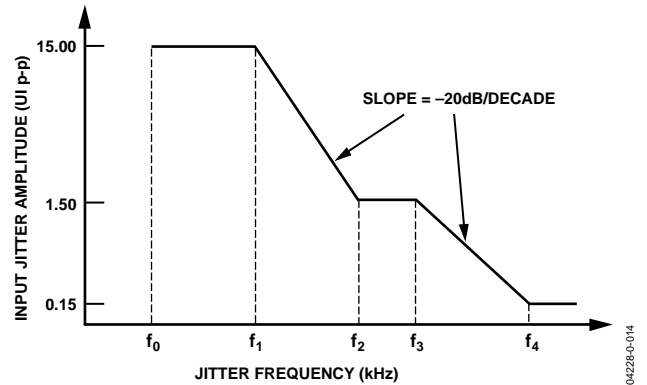
Figure 16. SONET Jitter Tolerance Mask
