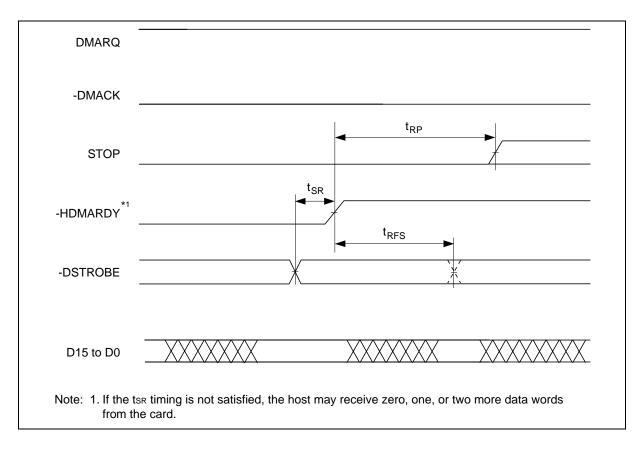
Timing of Host pausing an Ultra DMA data-in Burst
