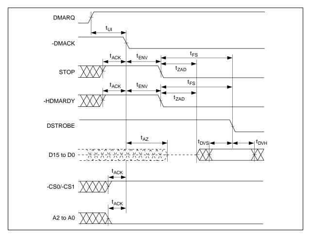
Timing of Sustained Ultra DMA data-in Burst
