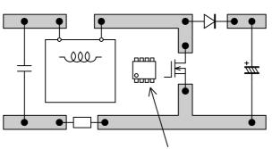
IC is arranged close to inductor or MOSFET
