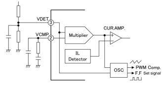
Fig.7 Block diagram for oscillator area
