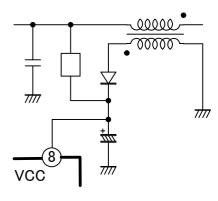
Fig.30 VCC pin circuit (1)
