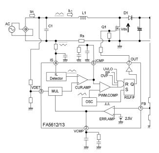
Fig.1 Block diagram of operating circuit
