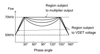
Fig.8 Oscillation frequency vs. phase angle
