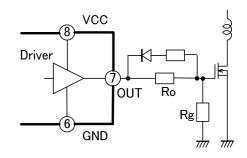
Fig.28 OUT pin circuit (3)
