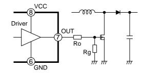
Fig.1 IS pin-connected filter resistance
