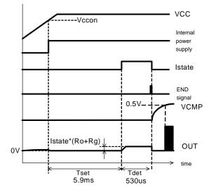
Fig.6 Frequency setting sequence
