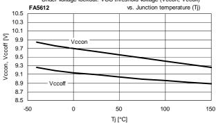
Under voltage lockout: VCC threshold voltage (Vccon, Vccoff)
