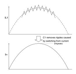
Fig.4 Power factor corrected waveform
