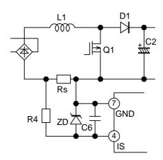
Fig.19 IS pin circuit (2)
