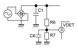
Fig.17 VDET terminal circuit
