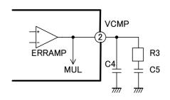
Fig.16 VCMP pin circuit
