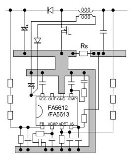
Fig.35 Example of advisable GND wiring
