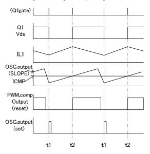
Fig.2 Waveforms of switching operation (outline)
