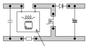
IC is arranged under inductor (or on immediately opposite side on circuit board)
