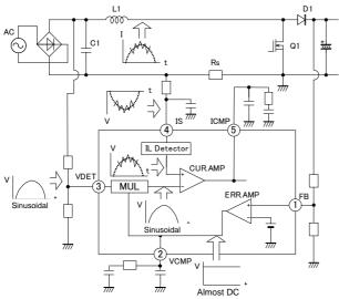
Fig.3 Aspects of waveforms at different parts
