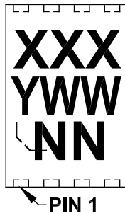
8-Lead DFN (2x3x0.9 mm)
