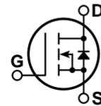
Power MOS 7™ is a new generation of low loss, high voltage, N-Channel enhancement mode power MOSFETS. Both conduction and switching losses are addressed with Power MOS 7™ by significantly lowering  $R_{DS(ON)}$  and  $Q_g$ . Power MOS 7™ combines lower conduction and switching losses along with exceptionally fast switching speeds inherent with APT's patented metal gate structure.
