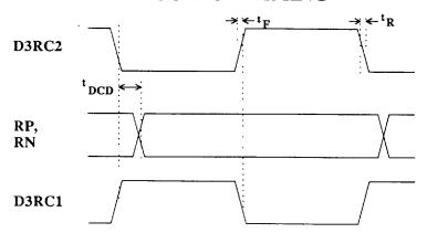
This figure illustrates the propagation delay of the data on the RP and RN pins with respect to the two clocks, D3RC1 and D3RC2. The only difference between the clocks is that one is the inverse of the other.
