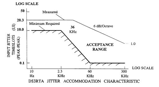
This jitter tolerance curve applies at the line input of the DS3RTA (pin 29, DS3IN1). The DS3RTA recovers clock, and outputs P and N rail data and clock in the presence of the pictured input jitter characteristic.
