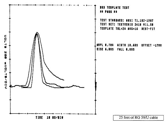
The peak amplitude of the pulse at the output of 25 feet of cable is 700 millivolts. The DS3RTA had the TXLEV lead (pin 35) at ground for the low level output (about 770 millivolts). The ANSI requirement at the DSX ranges from 850 to 360 millivolts. The observed amplitudes are within the required range for all cable lengths.
