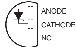
LP (TO-92/TO-226) PACKAGE (TOP VIEW)
