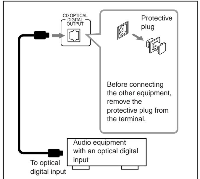
Connect an optical digital cord (not supplied) between the optical digital input terminal on the other equipment and the CD OPTICAL DIGITAL OUTPUT terminal.
