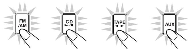
When you press the play button for a particular source (FM/AM, CD ▶/||, AUX, and TAPE ◀▶), the unit turns on, and the Powered Rolling Panel opens automatically (and the unit starts playing the source if it is ready — COMPU PLAY CONTROL).
