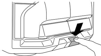
**2** Put in a recordable cassette, with the exposed part of the tape down.
