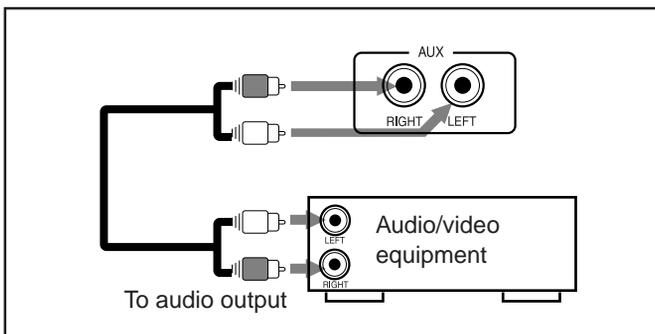
**For playing the other equipment through this unit,** connect between the audio output jacks on the other equipment and AUX jacks by using audio cords (not supplied).
