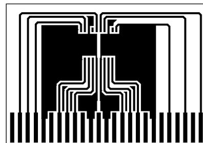
Fig 6. PCB used for thermal tests; heat sink area 400 mm²
