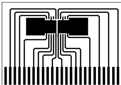
Fig 5. PCB used for thermal tests; heat sink area 200 mm²
