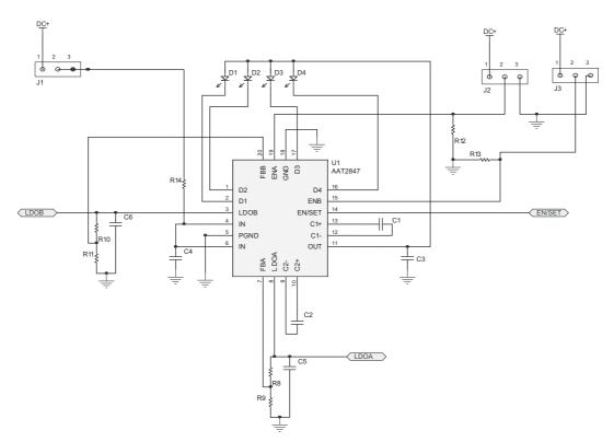
Figure 7: AAT2847 Section Schematic.
