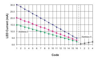
Figure 1: LED Current Control Profile.
