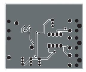
Figure 6: AAT2847 Evaluation Board Solder Side Layout.
