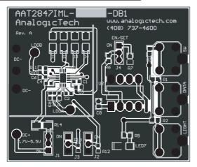
Figure 5: AAT2847 Evaluation Board Component Side Layout.
