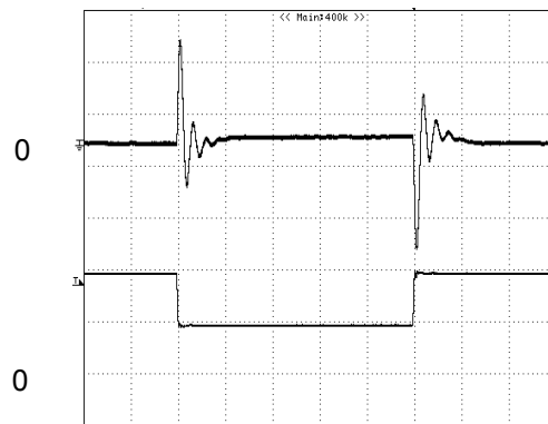
Figure 9: Output voltage response to step-change in load current (75%-50%-75% of I_{o, max} ; di/dt = 1.0A/\mu s ). Load cap: 100 \mu F tantalum capacitor and 1 \mu F ceramic capacitor. Top Trace: V_{out} (100mV/div, 200 \mu s /div), Bottom Trace: I_{out} (10A/div). Scope measurement should be made using a BNC cable (length shorter than 20 inches). Position the load between 51 mm to 76 mm (2 inches to 3 inches) from the module
