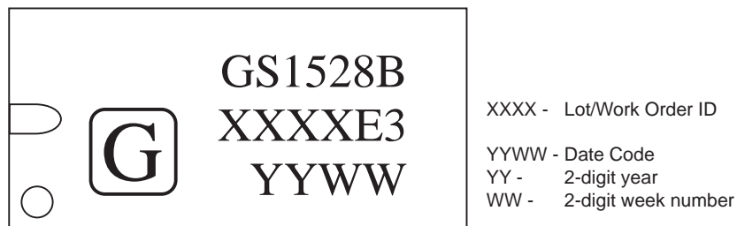
Figure 7-2: GS1528B Marking Diagram
