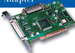
The LSI8953U Ultra2 SCSI host adapter is a low cost SCSI solution for any application needing to add a SCSI adapter.
