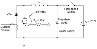
Fig. 8 - Unclamped Inductive Test Circuit
