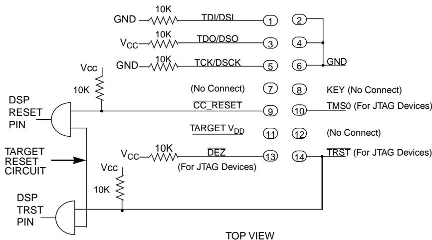
Figure 2-1. Target  $V_{DD}$  System JTAG/OnCE™ Interface Connector
