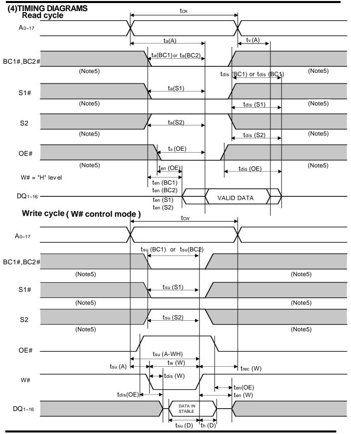
4194304-BIT (262144-WORD BY 16-BIT) CMOS STATIC RAM
