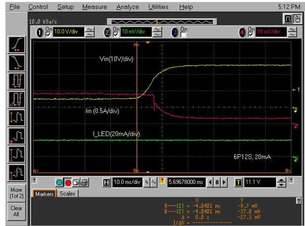
FIGURE 14. LINE REGULATION WITH V_{IN} CHANGE FROM 6V TO 26V, V_{IN} = 12V , 6P12S AT 20mA/CHANNEL
