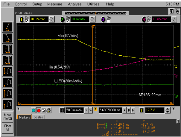
FIGURE 15. LINE REGULATION WITH V_{IN} CHANGE FROM 26V TO 6V FOR 6P12S AT 20mA/CHANNEL
