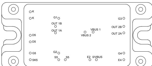
All multiple inputs and outputs must be shorted together
