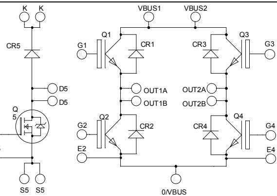
Full bridge top switches : Trench + Field Stop IGBT
