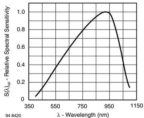
Fig. 2 - Relative Spectral Sensitivity vs. Wavelength
