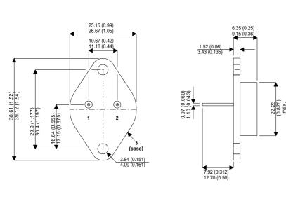
Bipolar NPN Device in a Hermetically sealed TO3 Metal Package.
