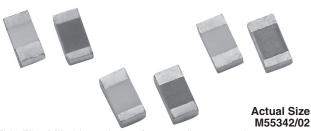
Thin Film Mil chip resistors feature all sputtered wraparound termination for excellent adhesion and dimensional uniformity. They are ideal in applications requiring stringent performance requirements. Established reliability is assured through 100 % screening and extensive environmental lot testing. Wafer is sawed producing exact dimensions and clean, straight edges.
