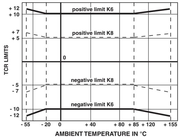
The temperature coefficient is guaranteed between - 20 °C to + 85 °C.
