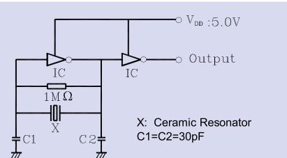
Parts shall be measured under a condition (Temp.: 20±15°C, Humidity: 65±20% R.H.) unless the standard condition (Temp: 25±3°C, Humidity: 65±10% R.H.) is regulated to measure
