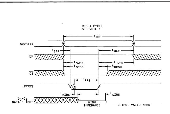
NOTE: Reset cycle is defined by the overlap of  $\overline{RS}$  and  $\overline{CS}$  for the minimum reset pulse width.
